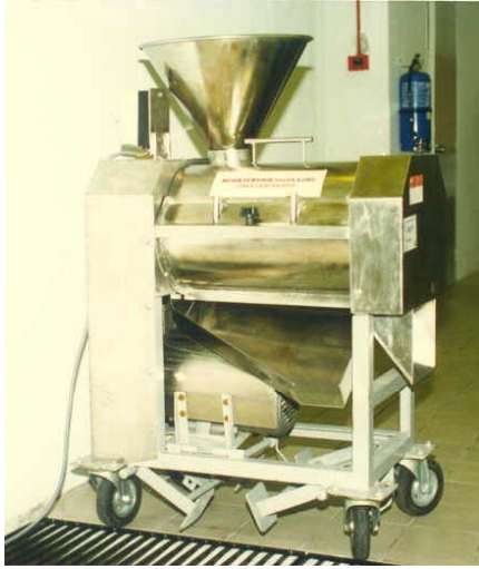
Locally fabricated cocoa depulper for pulp extraction
